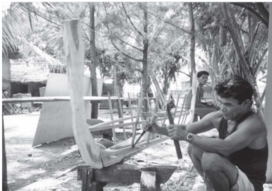
Construction of a small non-motorized banca.
